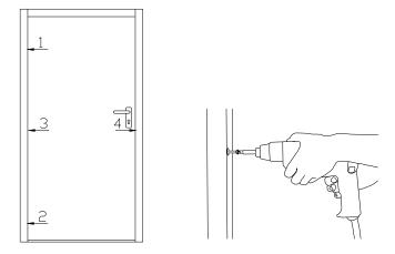
**5.** Using long countersunk frame fixings, first fix as shown, with 3 fixings in the hinge jamb and 1 in the lock jamb.
