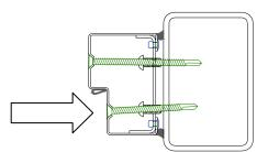
**8.** Open the door fully, then tighten the 2nd set of frame adjusters in the reveals.
