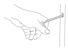
**3.** Tighten the six frame adjusters clockwise, with a 5mm ball-ended Allen key, until the ends of the spreader plates are flat against the wall.
