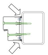
**11.** Apply mastic or flashings to seal frame to building. Fire rated doorsets must be sealed as shown, all round the frame, using either:
