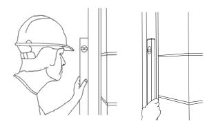
**4.** Ensure the frame is vertical in both planes, particularly the hinge jamb.
