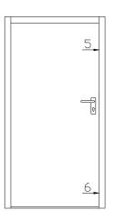
**7**. Close the door again, then fit the last 2 fixings into face 5 of the lock jamb.
